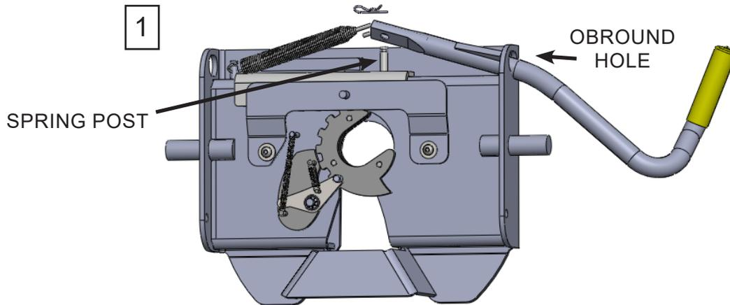
2. Detach the spring from the spring post and stretch hook inside handle so it reaches beyond the hole in the handle.
