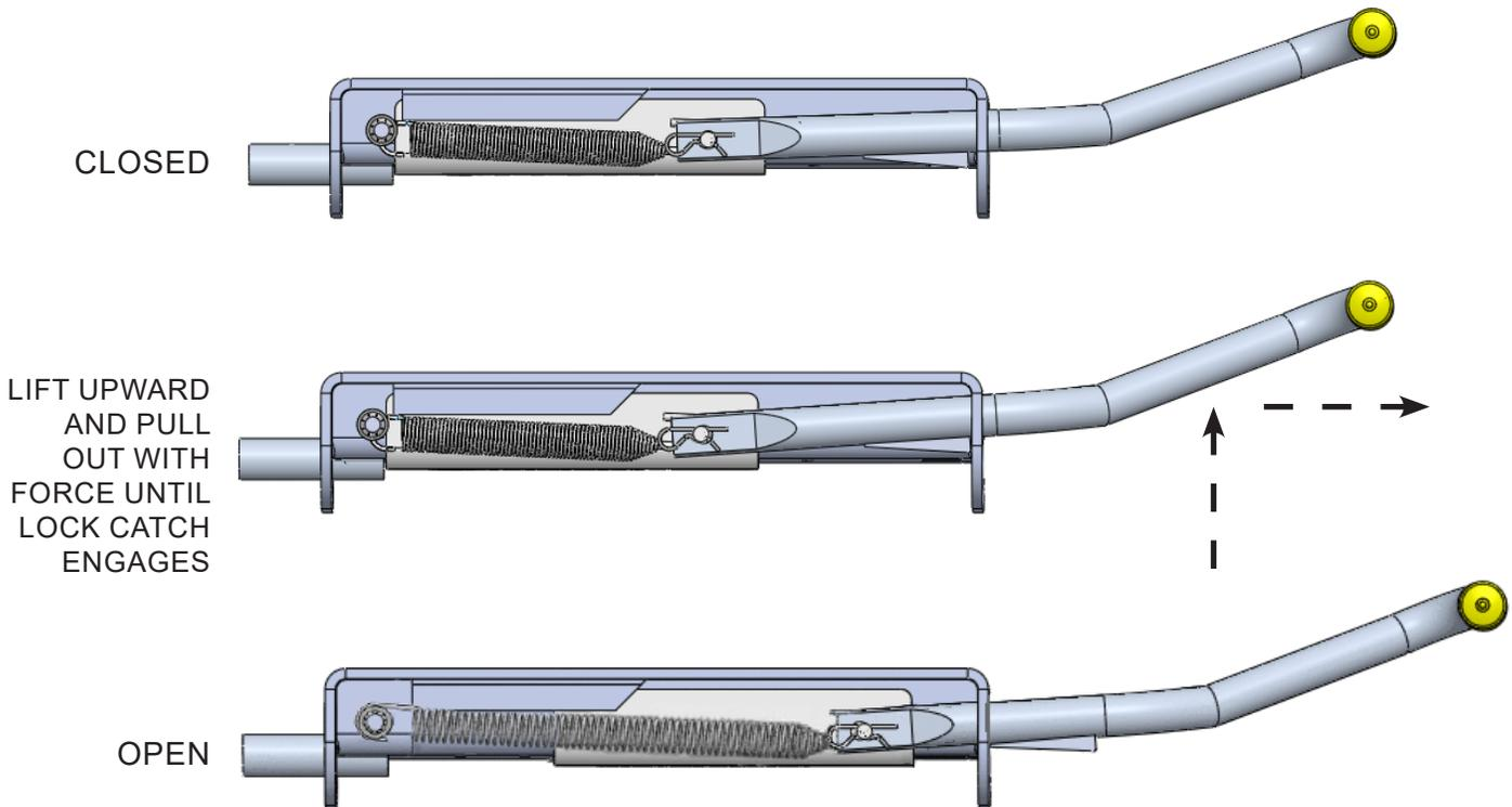
To discourage theft or pranksters, place a padlock through the obround hole above the Release Handle (see Illustration below).
