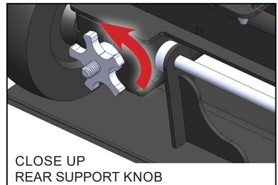
When the SuperGlide is removed and ready for storage, unscrew the (2) REAR SUPPORT KNOBS (FIG.B) and flip the REAR SUPPORT into the upward position (FIG. D) Lock in place by inserting the spring loaded Latch Pin into the slot in the REAR SUPPORT.
