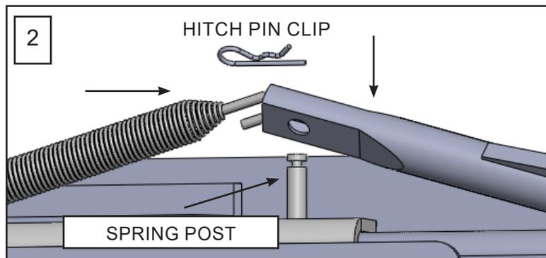
3. Bring the handle and spring down over the spring post and replace the hitch pin clip.
