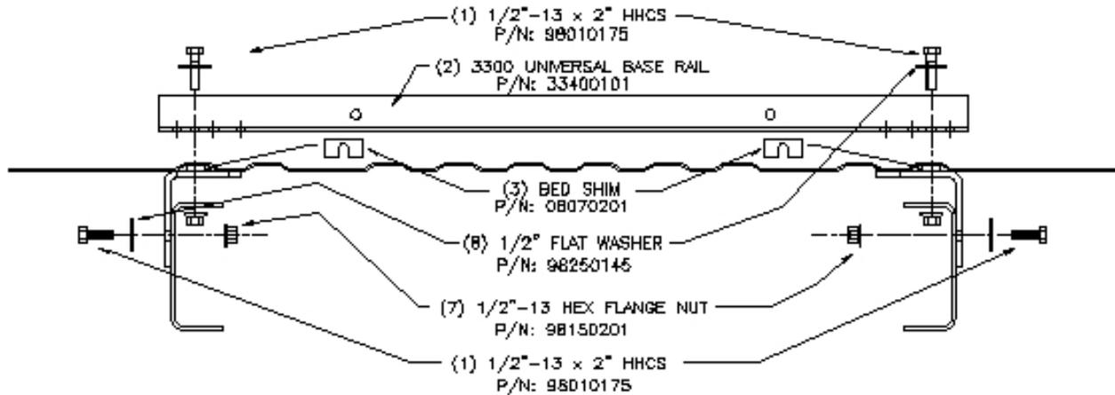
FASTENERS USED FOR BED HOLE LOCATIONS
